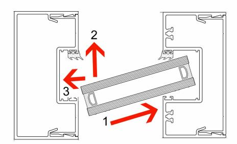
Once all the beads are in, it is time to fit the wedge gasket. We recommend fitting all 4 sides as a single piece, snipping the rear edges in the corner. This gasket is meant to be tight to prevent water ingress. If you are struggling try using hot soapy water to aid fitting.
