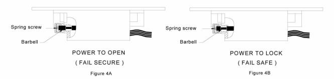
WARNING: Do not attempt to swivel the keeper while changing the function, this will damage the barbell mechanism.
