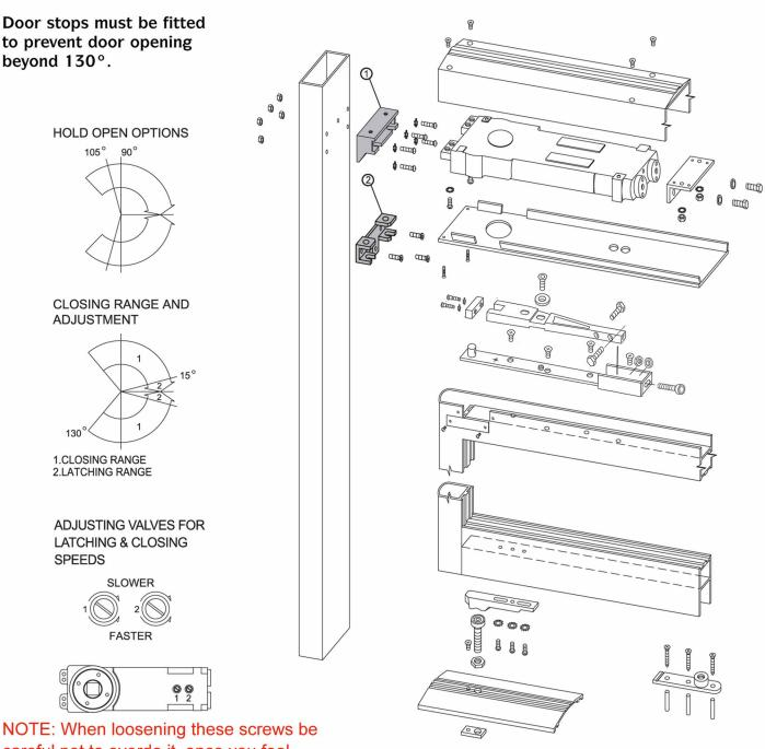
careful not to overdo it, once you feel resistance STOP. By forcing the screws looser you will damage the mechanism and it will fail.
