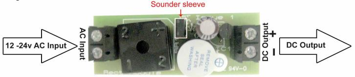
The sounder will buzz whenever an input voltage is present. If the sound is not required remove plastic sleeve by gently pulling off.
